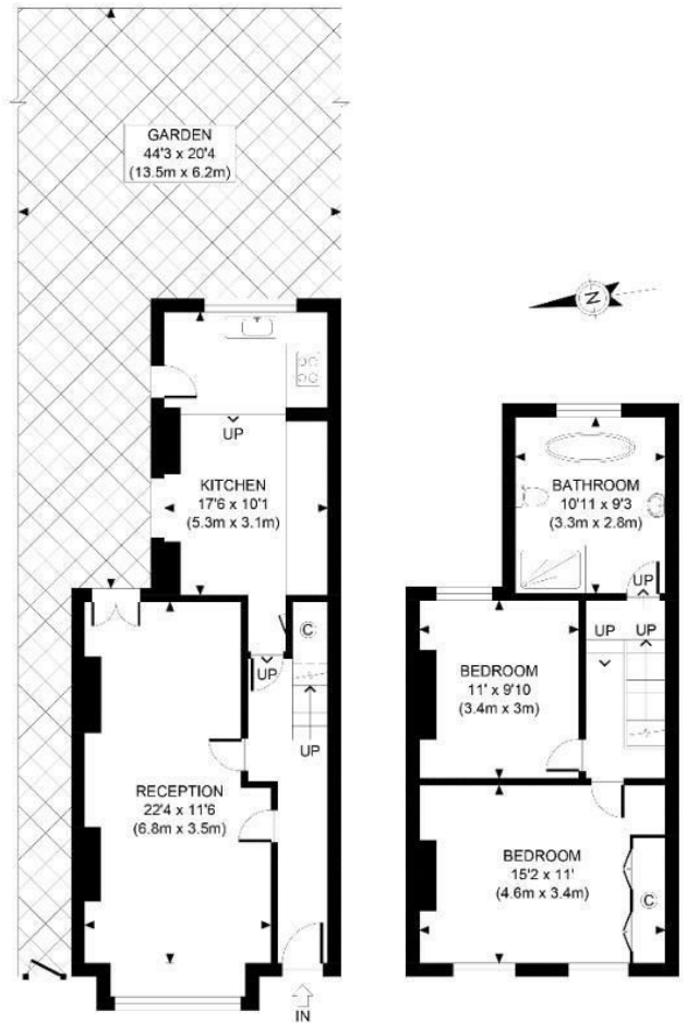
GROUND FLOOR GROSS INTERNAL FLOOR AREA 533 SQ FT FIRST FLOOR GROSS INTERNAL FLOOR AREA 445 SQ FT
